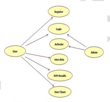
A use case diagram in the Unified Modelling Language (UML) is a type of behavioural diagram defined by and created from a Use-case analysis. Its purpose is to present a graphical overview of the functionality provided by a system in terms of actors, their goals (represented as use cases), and any dependencies between those use cases. The main purpose of a use case diagram is to show what system functions are performed for which actor. Roles of the actors in the system can be depicted.
