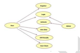
A use case diagram in the Unified Modelling Language (UML) is a type of behavioural diagram defined by and created from a Use-case analysis. Its purpose is to present a graphical overview of the functionality provided by a system in terms of actors, their goals (represented as use cases), and any dependencies between those use cases. The main purpose of a use case diagram is to show what system functions are performed for which actor. Roles of the actors in the system can be depicted.
