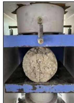
Fig 2 Specimen placed in CTM for Split-Tensile strength
