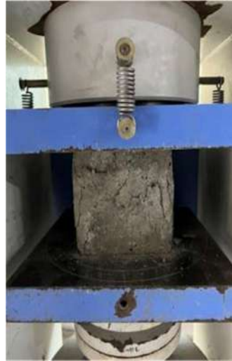
Fig no.1 Specimen placed in CTM for compressive strength
