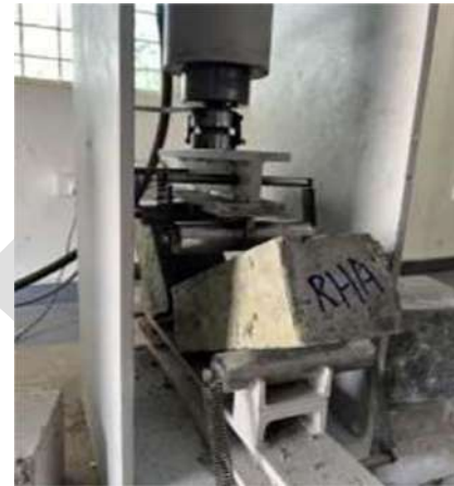
Fig 3. Specimen Flexure testing machine for Flexural strength.
