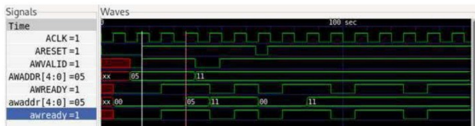
Figure 5.2.1: Address write channel with required signals
