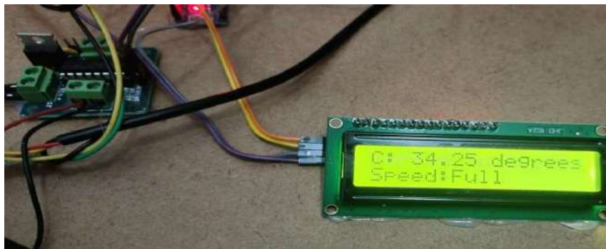
Fig 5.4 Shows that speed can be controlled based on the temperature and persons
