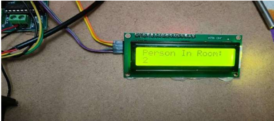
Fig 5.3 Shows that the IR sensor count the number of persons
