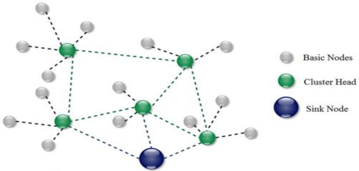
**Figure1. Basic Communication Structure of WSN**
