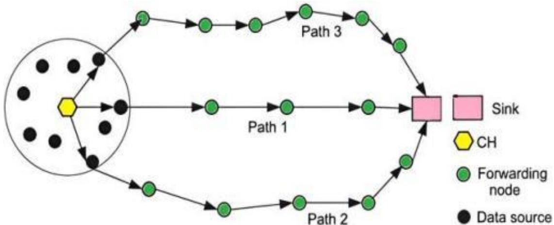
Figure 2. Various routing trails in WSN
