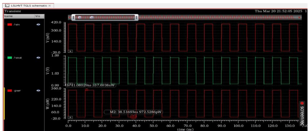
Fig 2: Power analysis of Transmission gate Level Shifter
