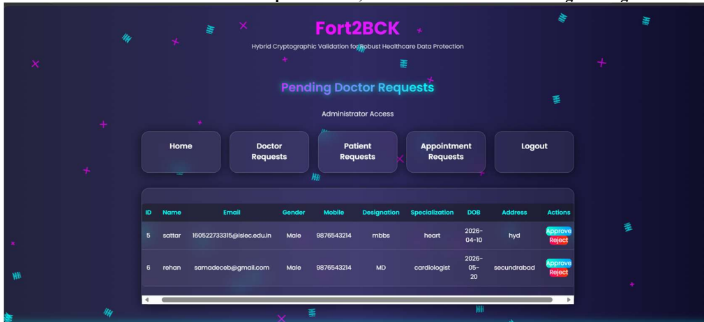
Fig. 3. Administrator Dashboard — Interface for managing pending doctor registration requests within the Fort2BCK system, showing applicant details such as ID, name, email, gender, mobile, designation, specialization, date of birth, and address, with options to approve or reject each request.
