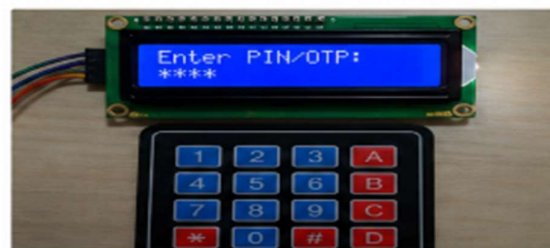
Fig 4.5: PIN/OTP Entry Interface using Keypad and 16x2 LCD Display
