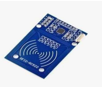
Figure 2: RFID reader Module
