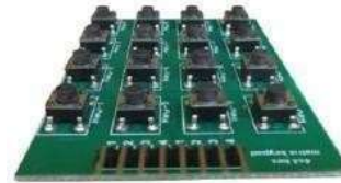
Figure 6: keypad (4x3 Matrix Keypad)
