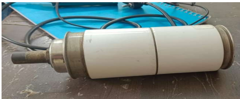
Fig 5: Vacuum Circuit Breaker(VCB)
