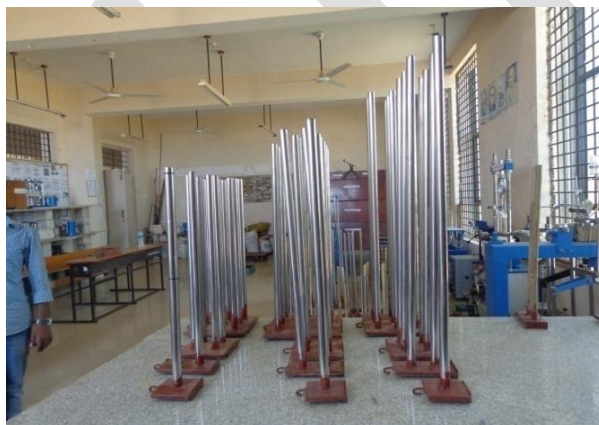
Fig.3. Different slenderness ratios pile groups of steel pipe materials models.
