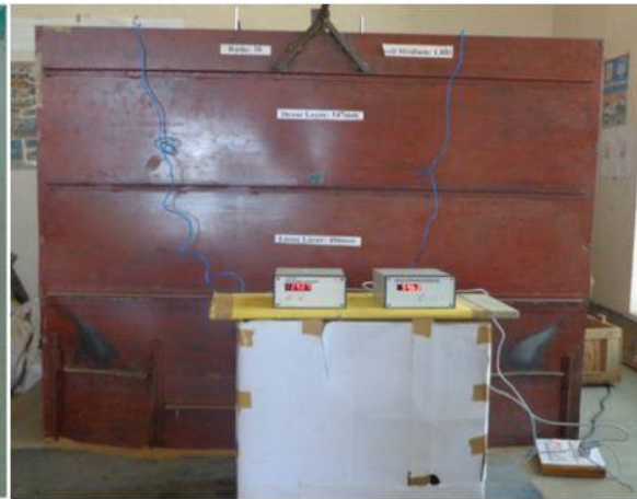
Fig.8. Setup of applying lateral loads and view of nine LVDT display units.
