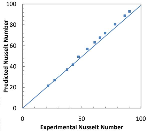
**Fig.8 Comparison of predicted tube side Nusselt number by eq. 10 and experimental Nusselt Number for square coiled tube**
