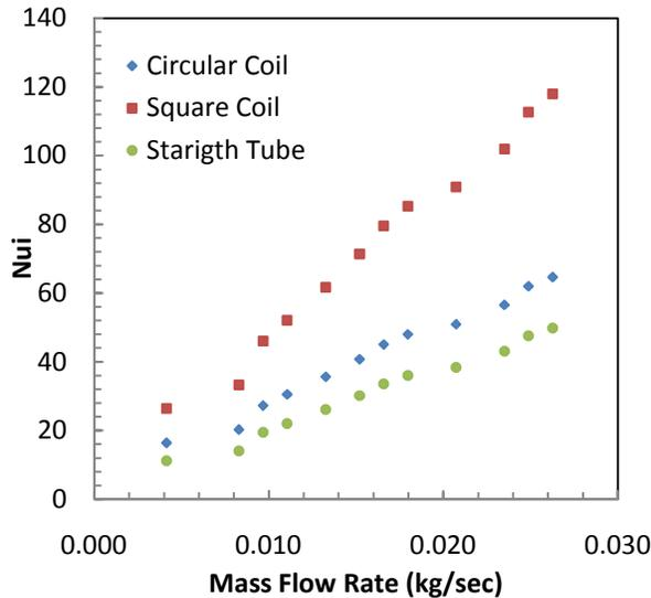
Fig. 5 Variation of inner Nusselt Number with various mass flow rate into various coil geometry
