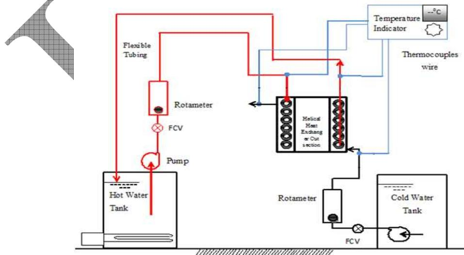
**Fig. 2 Experimental Setup of Helical coil heat exchanger**
