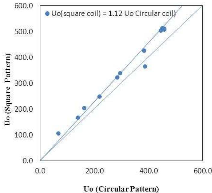
**Fig. 10 Comparison of tube side overall heat transfer coefficient of circular and square coiled heat exchanger**
