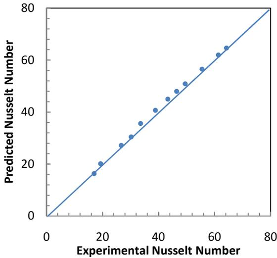
**Fig.7 Comparison of predicted tube side Nusselt number by eq. 9 and experimental Nusselt Number for circular coiled tube**
