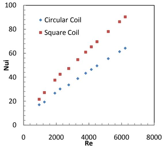
Fig. 6 Variation of inner Nusselt Number with Reynolds number for circular and square helical coil geometry
