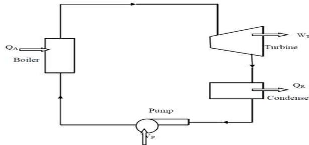
**Fig 1: Simple Rankine Cycle**
