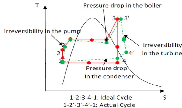
**Fig 3: Deviation of Rankine cycle**
