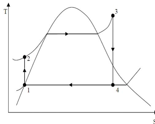
**Fig 2: T-S Diagram for simple rankine cycle**
