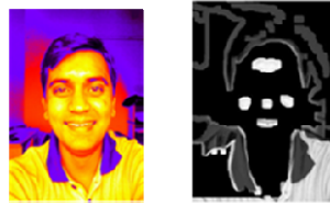
Figure 3 a). Thermal image of "Happy" Expression of human. b) Eigenface of thermal image.
