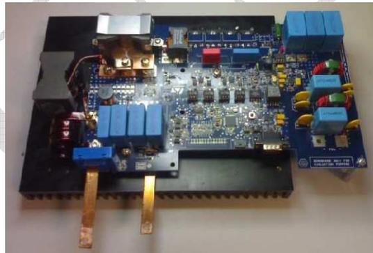
Fig. 5: 1.5kW DC-DC converter
